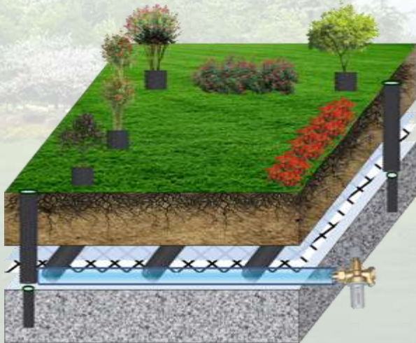
AMP-Arched Mesh Pipe-Green Roof Sub-Irrigated Raised System
