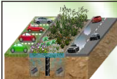
Rain Garden Irrigation & Drainage
