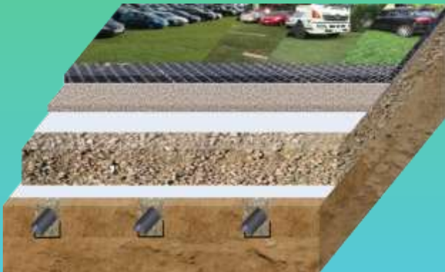
Permeable Green Pavement
