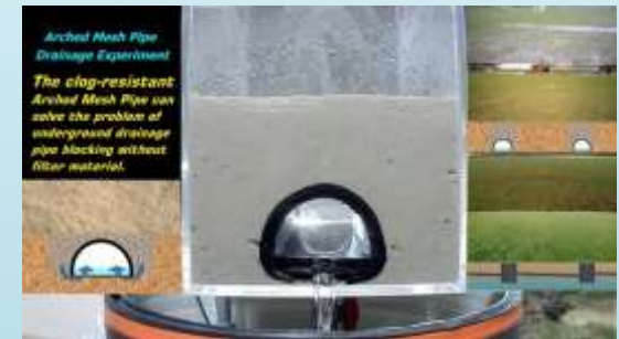
SMPS-Arched Mesh Pipe System Subsurface Drainage Experiment
