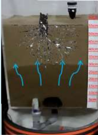
Capillary Action Subsurface Irrigation
