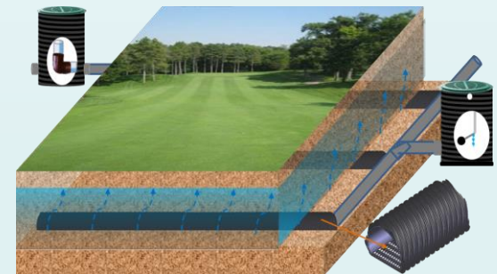
Fairway irrigation & drainage
