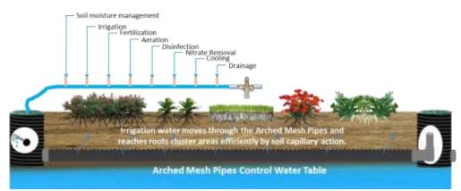
Irrigation: Irrigation water through AMP-Arched Mesh Pipe into the soil, using soil capillary action, supply to the Root cluster area.
