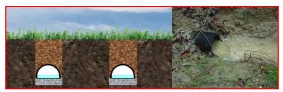
The underground irrigation drainage system uses capillary action to irrigate from the ground up, the ground is moist, the surface is dry, so its weeds are not easy to grow, and because the surface is dry, the air environment is also very dry, so compare There is no problem with pests and diseases.
