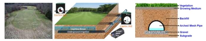
Arched Mesh pipe underground irrigation drainage system (AMPS) water non-pressurization and gravity-driven management system, irrigation water infiltrated into the soil through the infiltration network pipe, the use of soil capillary action, replenish water to the root group area. It can save 50% of irrigation water, increase fertilizer efficiency by 40%, and reduce irrigation manpower by 60%.
