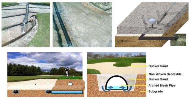
AMP-Arched Mesh Pipe using water infiltration and soil gravity separation principle, such as non-woven filter without clogging is not easy to produce, ecological engineering construction, long life, is to solve the problem of clogging the underground drainage pipe through the best set of drainage materials.
