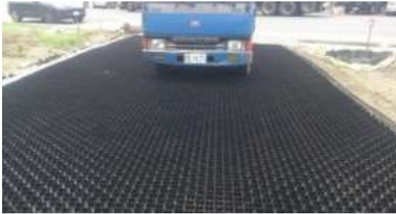
Grass grid loading test
